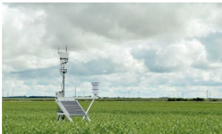
This Crop Sentry station was installed in a pea field in the spring. It is one of 15 sensors deployed across the farm in 2024.
